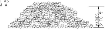
SECTION FRONT VIEW NOTE: BRUSH BARRIER(S) WILL BE INCLUDED IN PAYMENT FOR CLEARING & GRUBBING. BRUSH BARRIER DETAILS (FOR USE IN RURAL AREAS)
