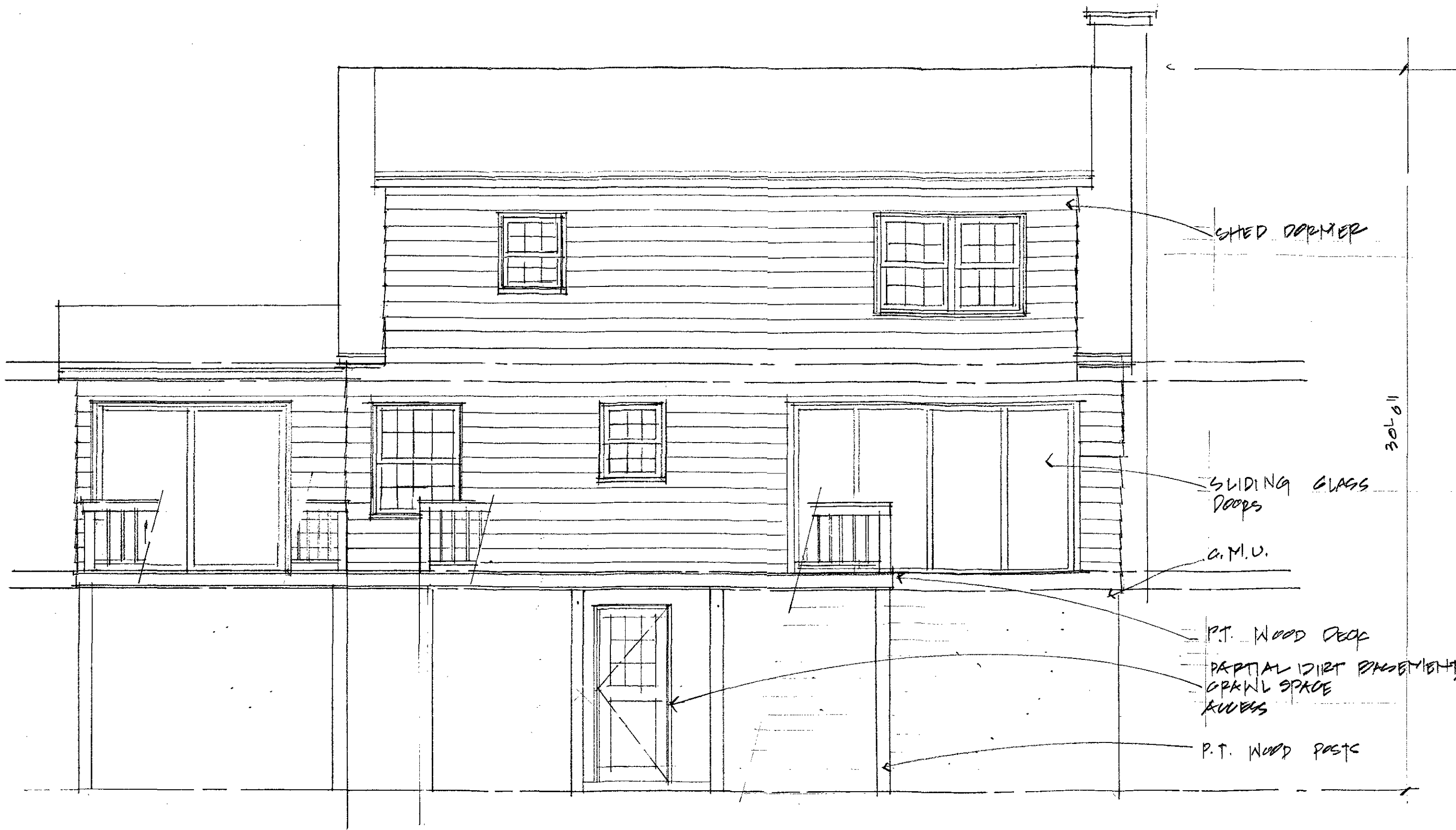
2 EXISTING REAR (EAST) ELEVATION A-1.3 1/4" = 1'-0"
