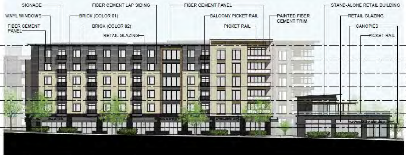
ELEVATION 2 - BUILDING A (BRIARCLIFF RD)
