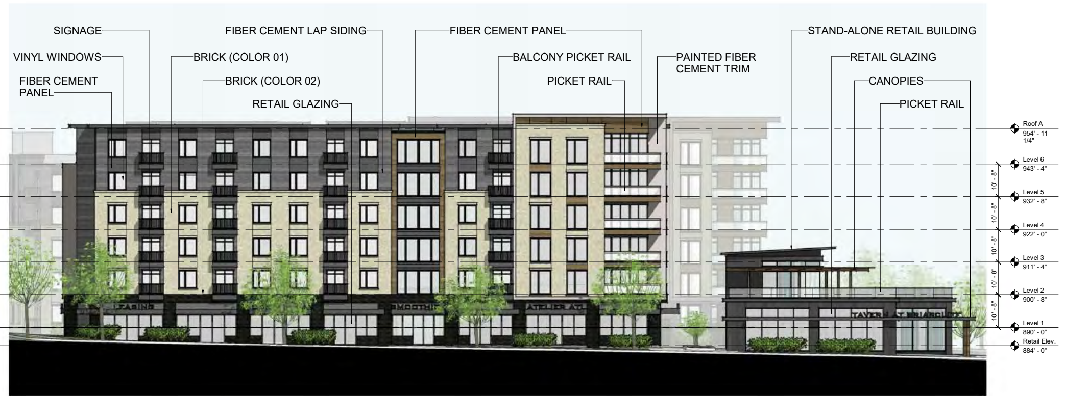
ELEVATION 2 - BUILDING A (BRIARCLIFF RD)
