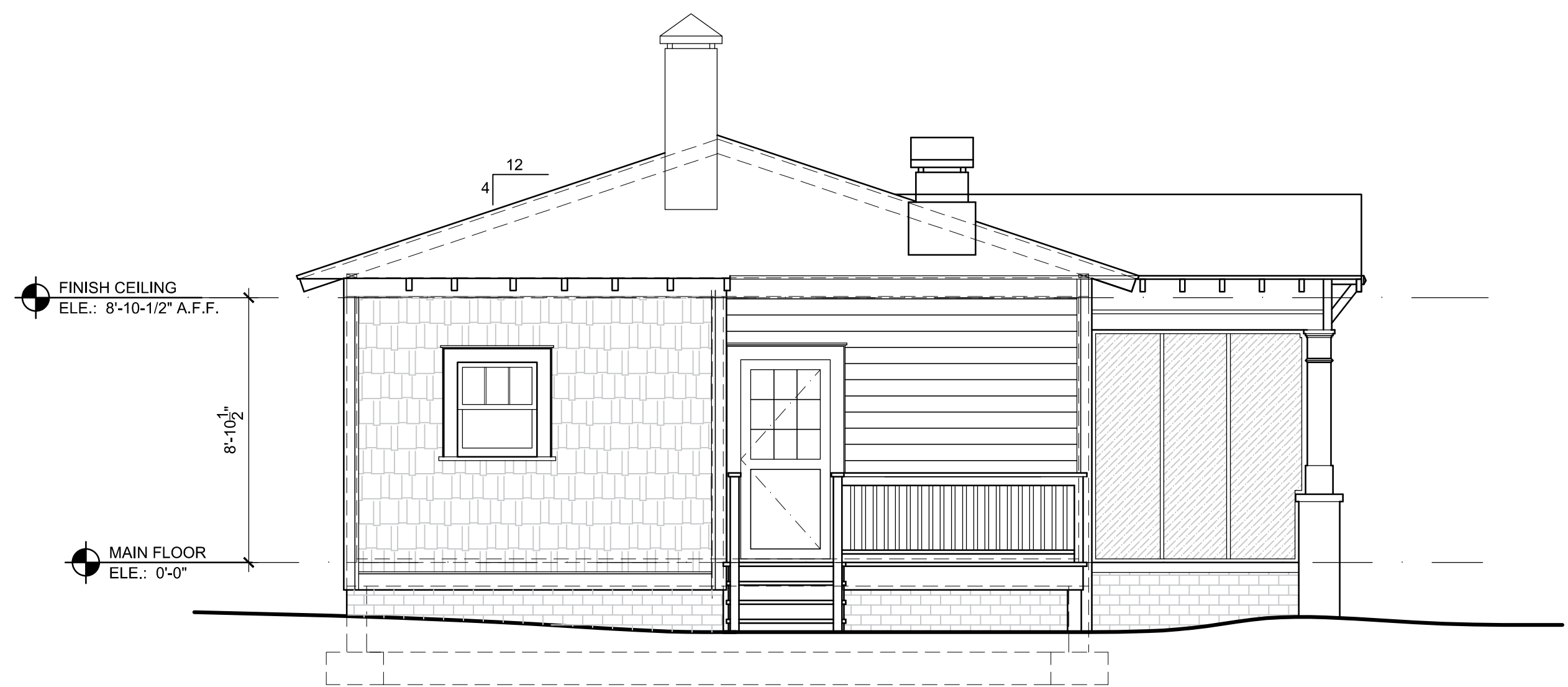
2 EXISTING EXTERIOR ELEVATION - REAR SCALE: 1/4" = 1'-0"
