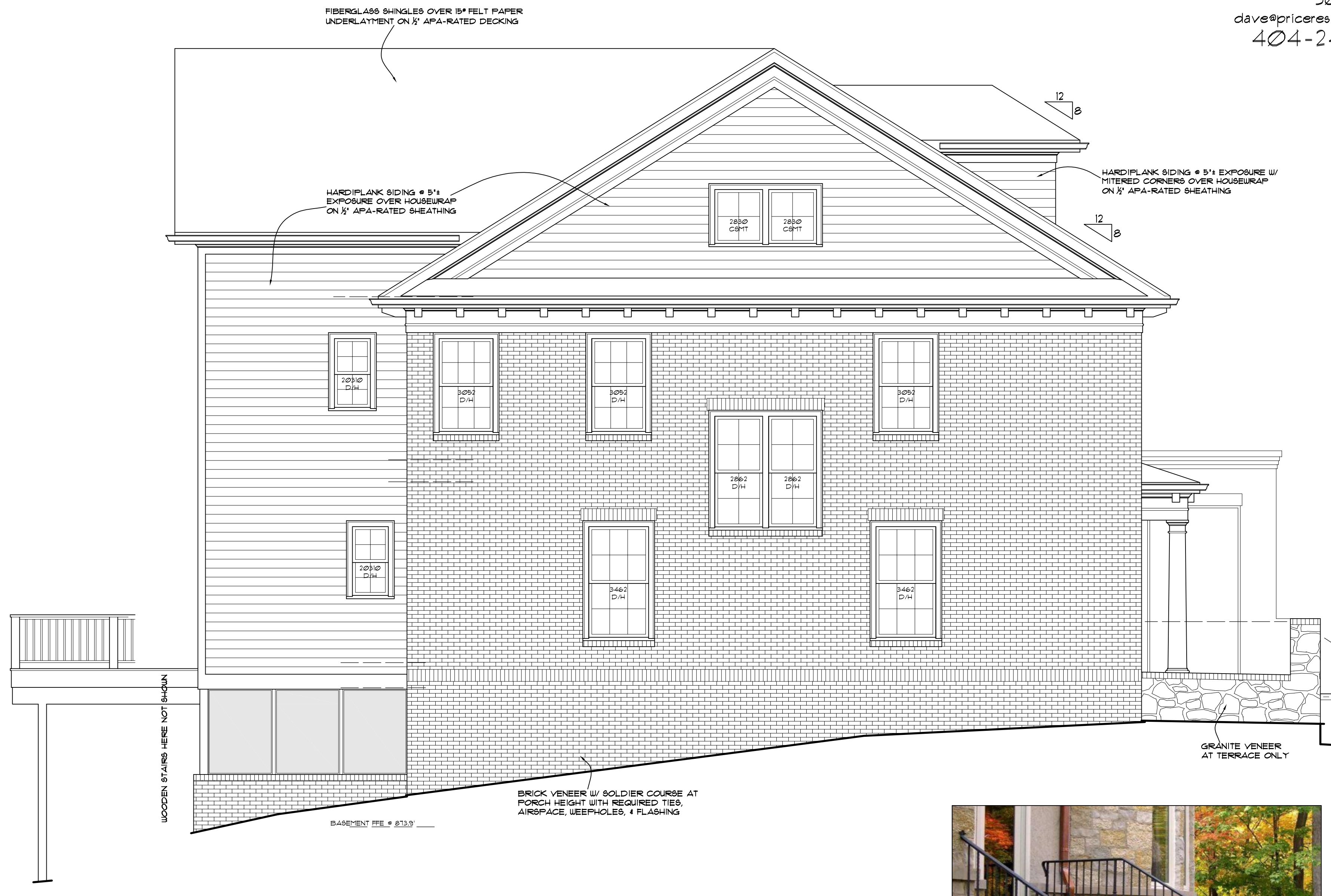
LEFT SIDE ELEVATION SCALE: 1/4" = 1'-0"
