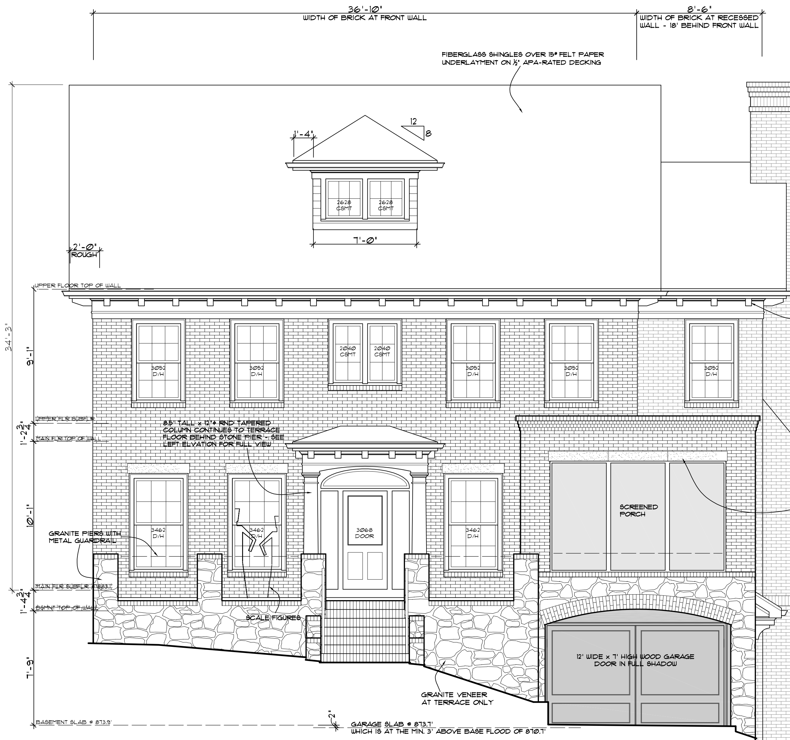
FRONT ELEVATION SCALE: 1/4" = 1'-0"
