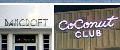
**OPTION 6A:** Traditional Neon in a Channel with a Clear Acrylic Face Plate
