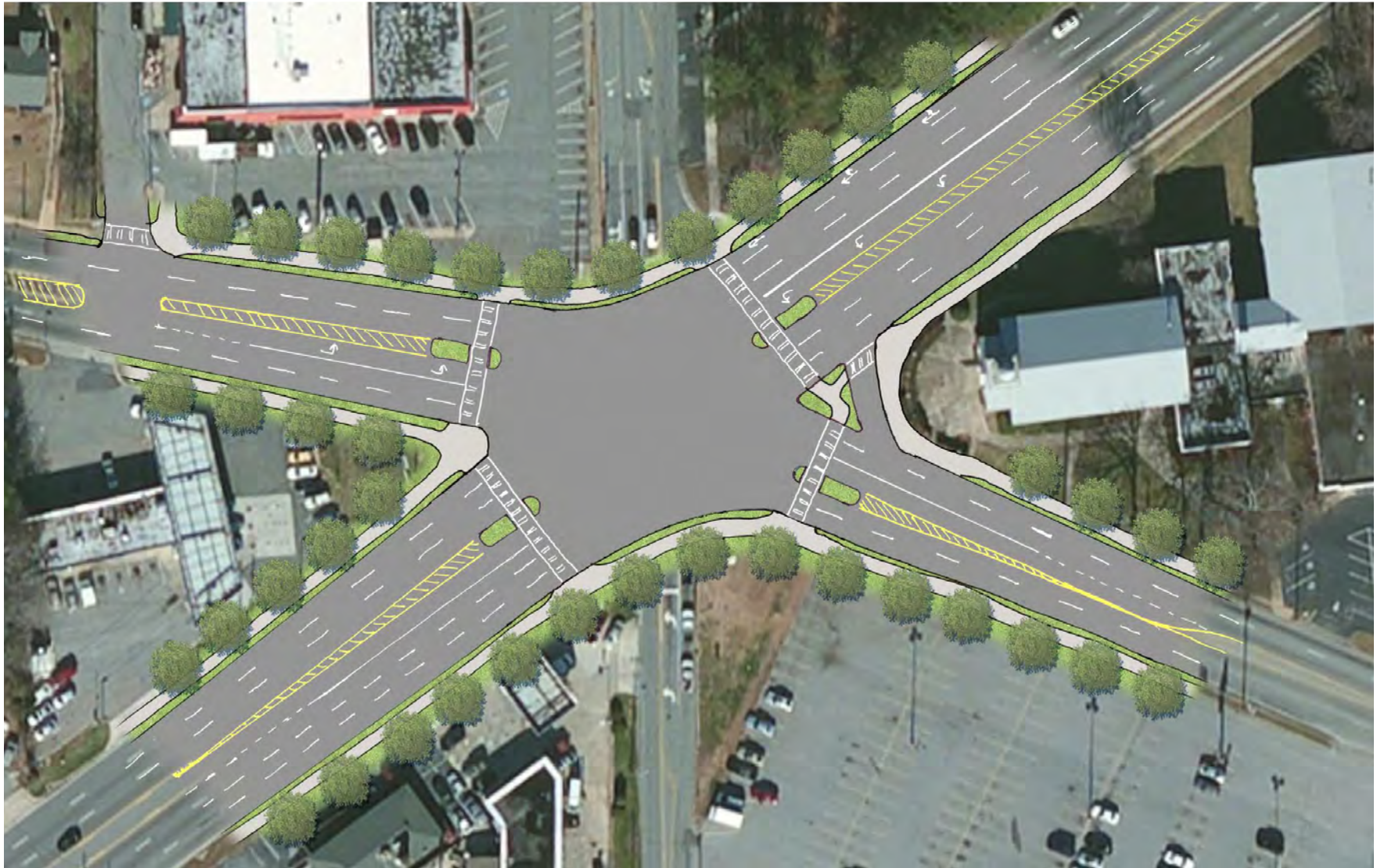
Figure 4vv: An option for improvements to the six-way intersection includes pedestrian refuge islands and closing off a portion of Medlock Street to automobile traffic.
