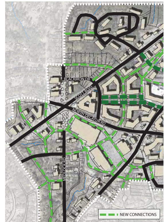
Figure 4uu: Alternative connectivity to Scott Boulevard and North Decatur Road from the surrounding community is key to closing off a portion of Medlock Road to vehicular traffic.
