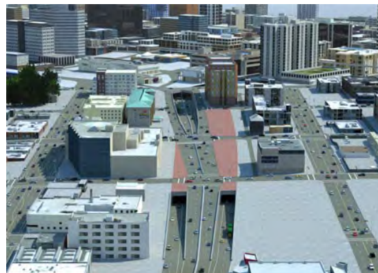
Figure 4ss: Example of Option 2: Bridge Through-traffic under, with local traffic remaining at grade.
