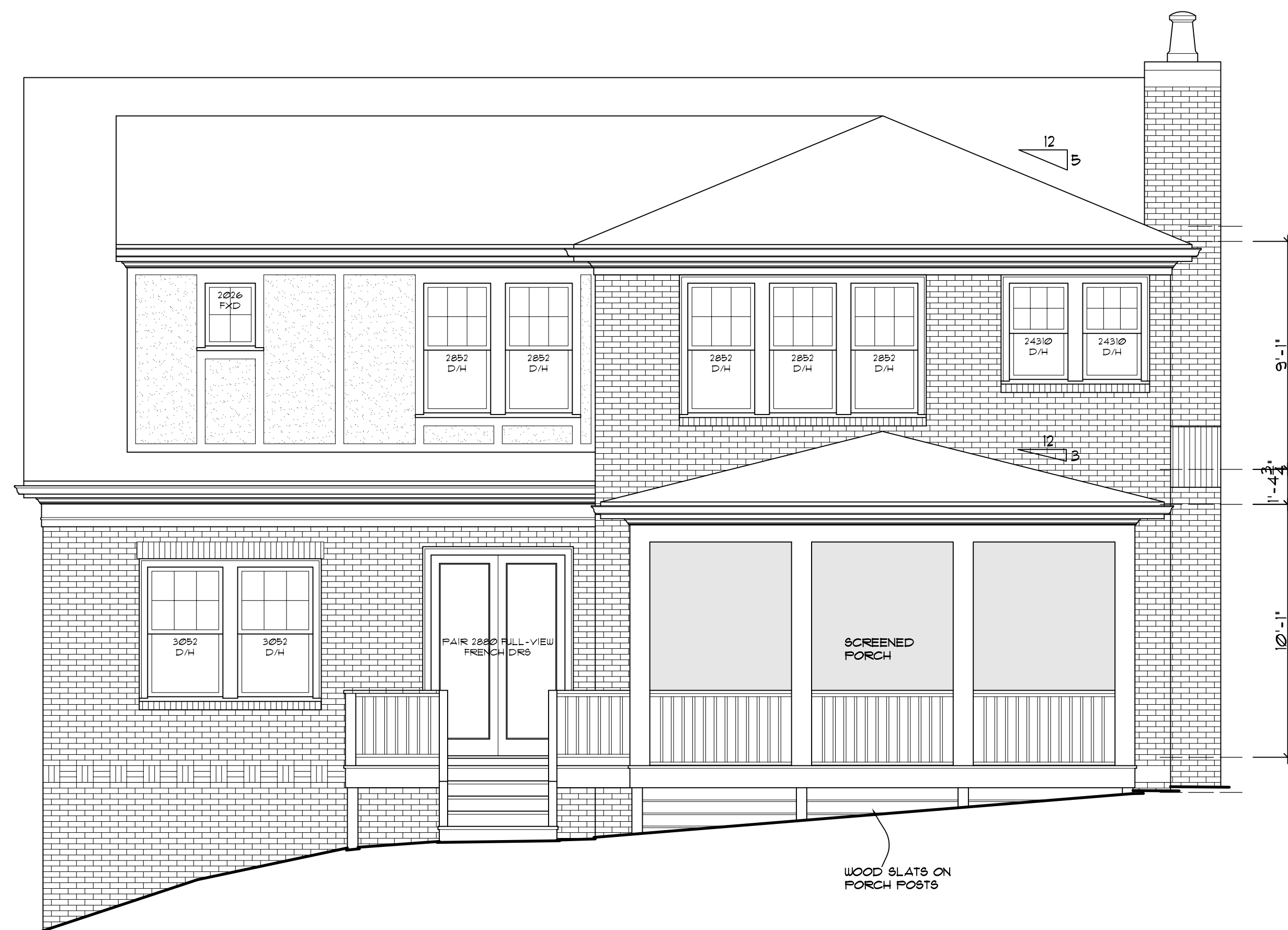
REAR ELEVATION SCALE: 1/4" = 1'-0"
