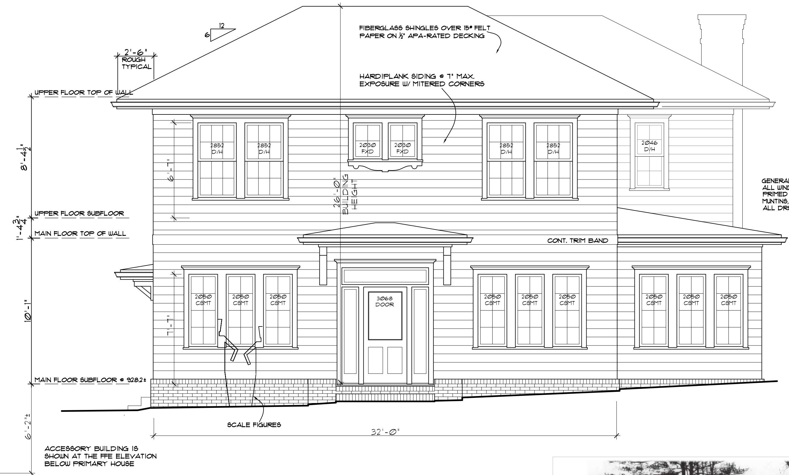
PRIMARY FRONT ELEVATION SCALE: 1/4" = 1'-0"
