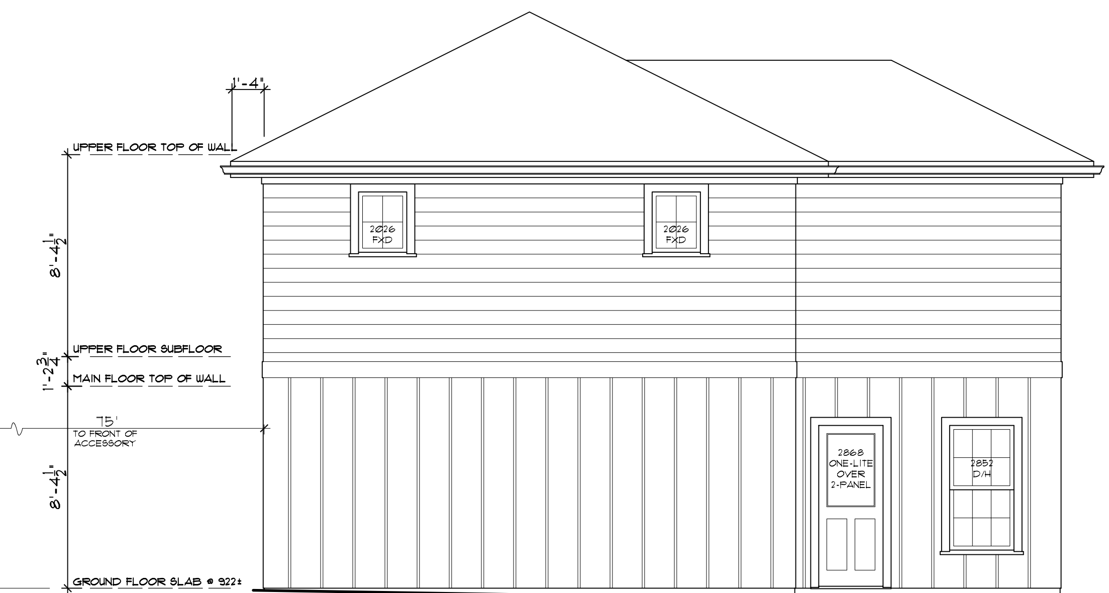
GARAGE/ADU. RIGHT ELEVATION SCALE: 1/4" = 1'-0"
