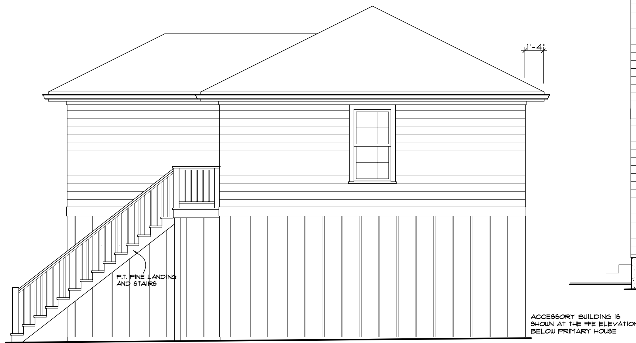
GARAGE/ADU. LEFT ELEVATION SCALE: 1/4" = 1'-0" FRONT FACE OF ACCESSORY IS 15' BEHIND REAR FACE OF PRIMARY HOUSE
