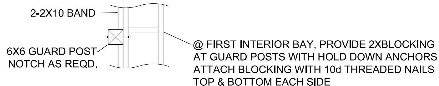
PLAN OF GUARD POST ATTACHMENT TO SIDE BAND
