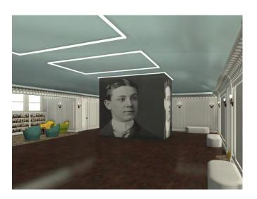
IMG 311-3: Interior rendering showing restored space. Non-historic elevator shaft to remain in current location. Ornamental cove crown moulding is still intact for restoration. The majority of original wall panel trim is also intact.
