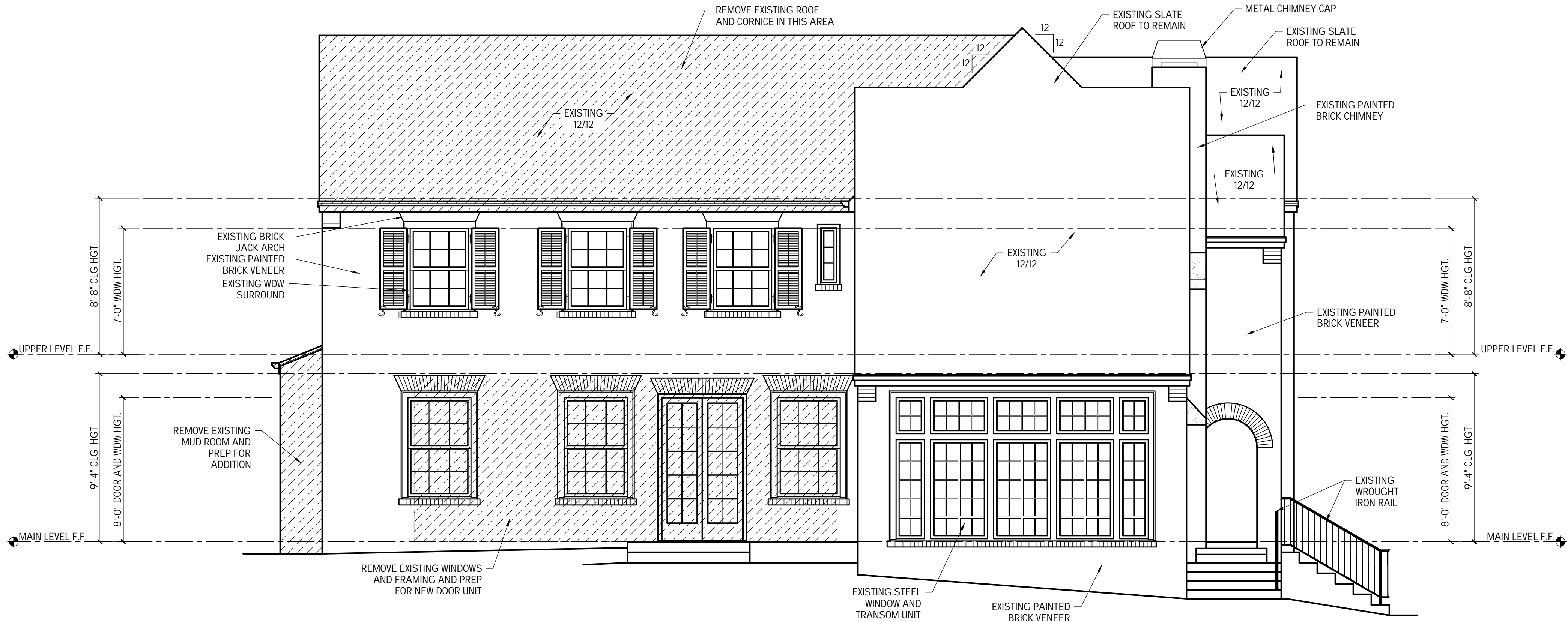
1 X_301 AS-BUILT / DEMO LEFT ELEVATION SCALE : 1/4"=1'-0"
