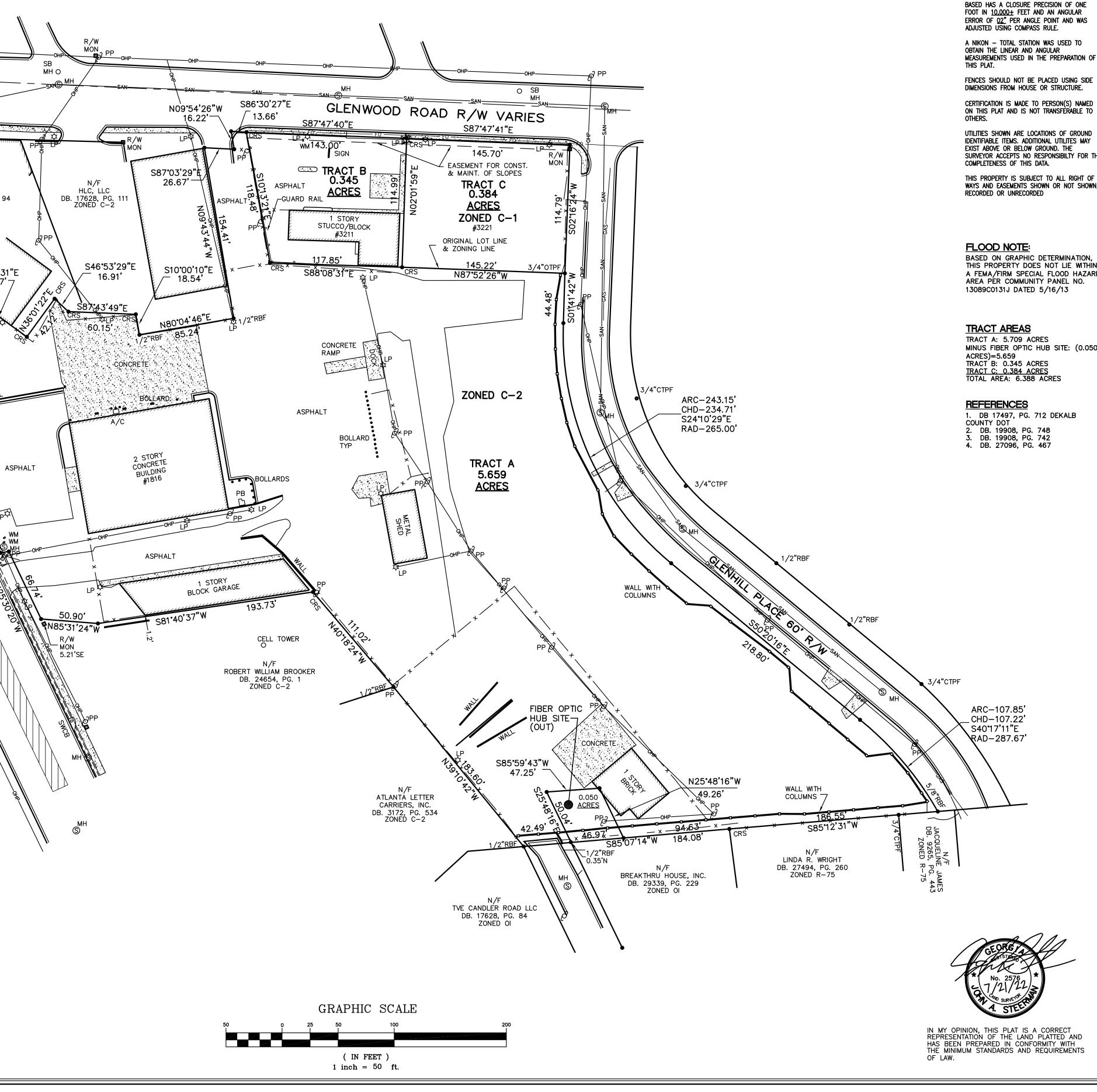
SURVEY NOTES: TRACT A THIS PLAT HAS BEEN CALCULATED FOR CLOSURE BY LATITUDES AND DEPARTURES AND IS FOUND ACCURATE TO WITHIN ONE FOOT IN <u>248.632</u> FFFT
