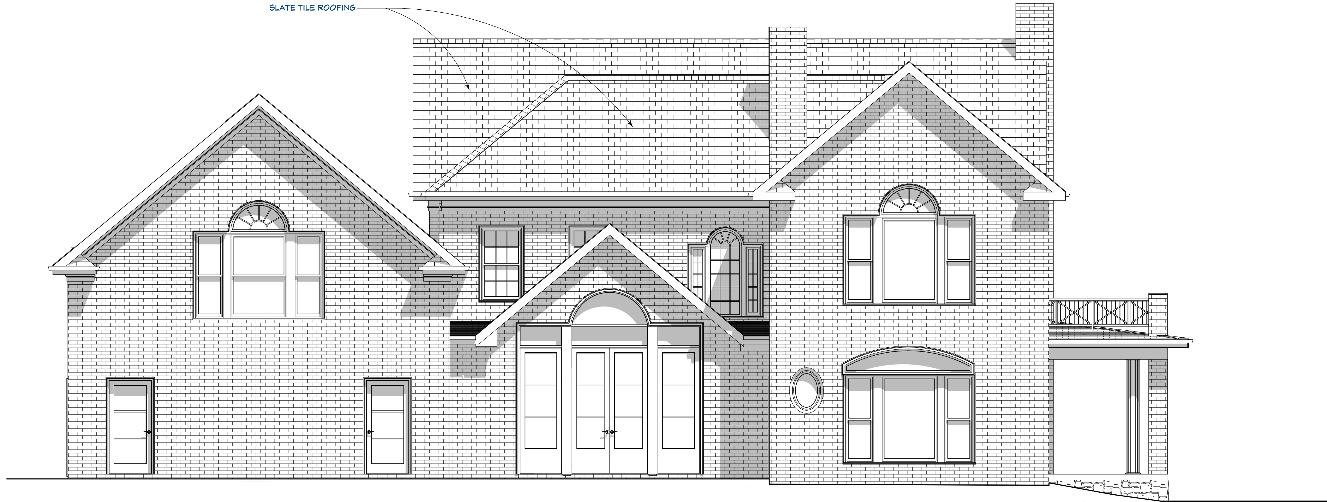
1 A4 AS-BUILT RIGHT ELEVATION SCALE= 1/4"=1'-0"
