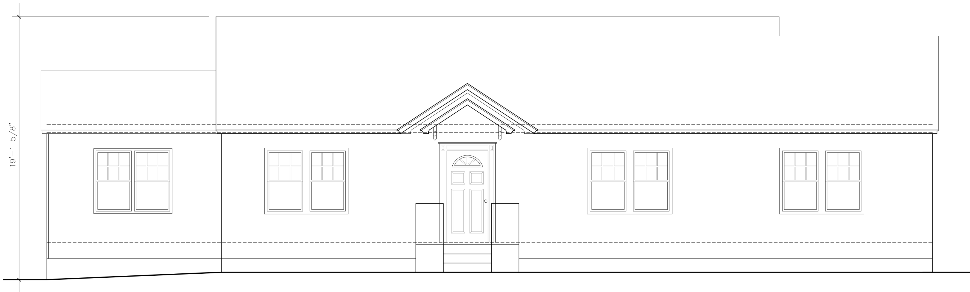
1 EXISTING FRONT ELEVATION SCALE: 1/4" = 1'-0"
