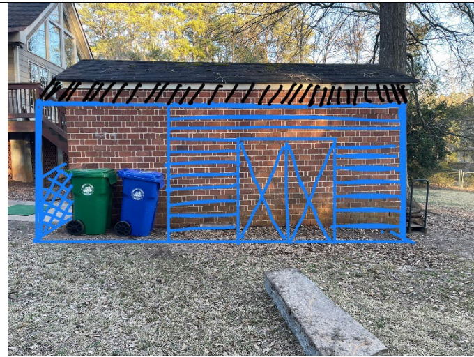
Figure 21. Side view schematic of proposed lean-to shed and waste container storage area. Shed constructed on right, open storage area on left with common roof.
