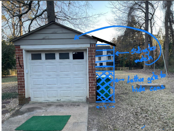
Figure 21. Side view schematic of proposed lean-to shed and waste container storage area. Shed constructed on right, open storage area on left with common roof.
