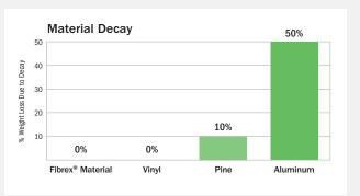
With Fibrex composite material, a special polymer formulation surrounds and coats each wood fiber in the manufacturing process, providing exceptional resistance to rot and fungal growth. Renewal by Andersen's windows, made with Fibrex composite material, never need scraping or painting because they are warranted not to flake, rust, blister, peel, crack, pit, or corrode.¹
