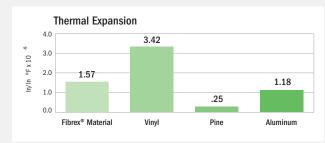
Fibrex composite material is durable and reliable, and – like wood, fiberglass, and aluminum – it expands and contracts very little. However, vinyl can expand and contract significantly. Vinyl may cause cracks, bowing, and air or water leaks. Windows made of Fibrex composite material will perform better in winter and summer than windows made of vinyl.
