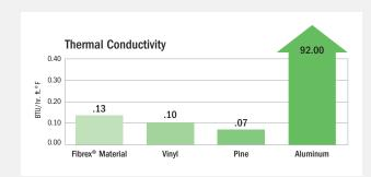
Fibrex composite material has excellent insulating properties on par with wood, vinyl, or fiberglass. Aluminum, on the other hand, transfers heat out of your home and allows outdoor temperatures to chill window areas inside. Fibrex composite material insulates about 700 times better than aluminum.
