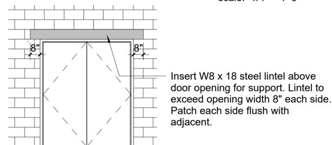
Insert W8 x 18 steel lintel above door opening for support. Lintel to exceed opening width 8" each side. Patch each side flush with adjacent.
