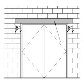
Insert W8 x 18 steel lintel above door opening for support. Lintel to exceed opening width 8" each side. Patch each side flush with adjacent.
