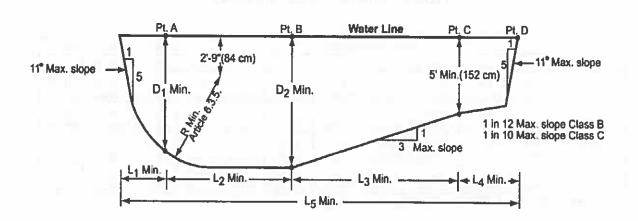
Figure 1 – Construction dimensions for water envelopes for Class B and Class C pools
