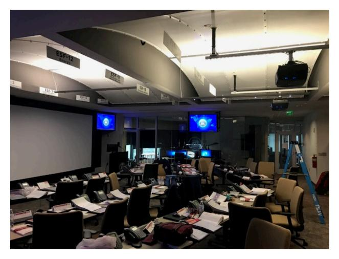
Projector Information X panel Controlled Crestron Pro 3 Processor Mounted Fixed Brackets Height to mounts 116" Distance from screen 286" Aspect Ratio 16 x 9 Picyure size 148" x 77" No on current code
