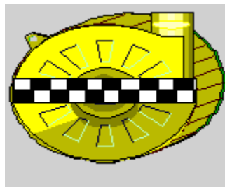
Figure 8-13 HMI Blower and Conveyor Graphics (Red = Stopped, Green = Running, Blinking Yellow = Alarm)
