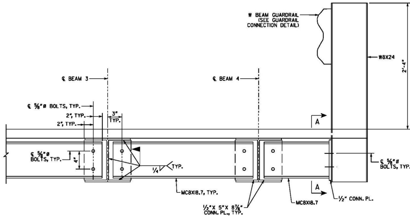
**GUARDRAIL AND DIAPHRAGM DETAIL**
