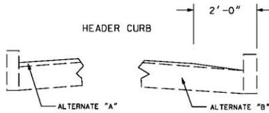
NOTE: METHOD OF FEATHERING OF PAVEMENT EDGE. (ALTERNATE A OR ALTERNATE B) SHALL BE DETERMINED BY THE ENGINEER. UNDER NORMAL CONDITIONS ALTERNATE A SHALL BE USED FOR FEATHERING UNLESS RESURFACING HAS REDUCED THE "EFFECTIVE HEIGHT" OF THE EXISTING CURB. IN THIS EVENT ALTERNATE B SHALL BE USED.
