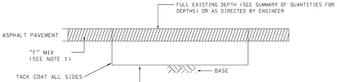
PATCHING SHALL BE ACHIEVED WITH "F" MIX (9.5mm) OR BINDER (19mm) IN COMPACTED 2" LIFTS AS DIRECTED BY ENGINEER ALL PATCHES SHALL BE A MINIMUM TWO INCHES IN DEPTH PATCH OUT PAVEMENT AREAS MARKED OUT BY THE ENGINEER
