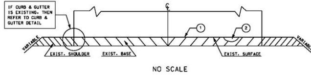
REQ'D ① 165 LBS PER SQ. YD. ASPH. CONC. "F" MIX (9.5mm) or "E" MIX (12.5mm) SUPERPAVE. TYPE II, BLEND 1, INCL. BITUMIN & H LIME, AS DIRECTED BY ENGINEER
