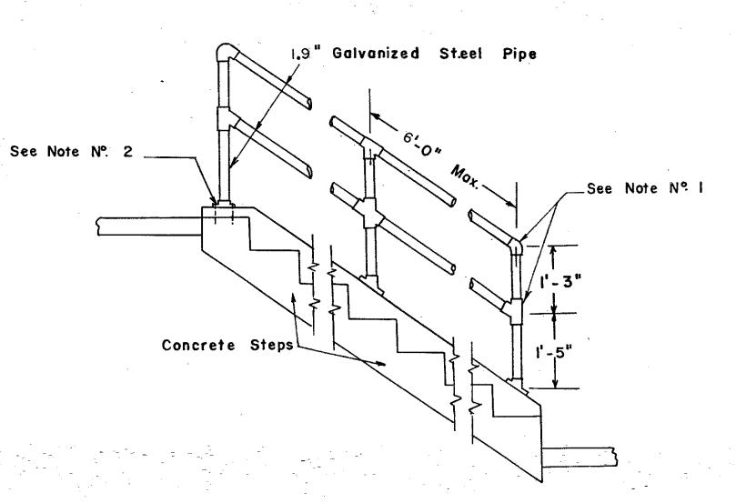
NOTE: PIPE, FITTINGS, FLANGES AND BOLTS SHALL BE OF AN APPROVED STANDARD TYPE.
