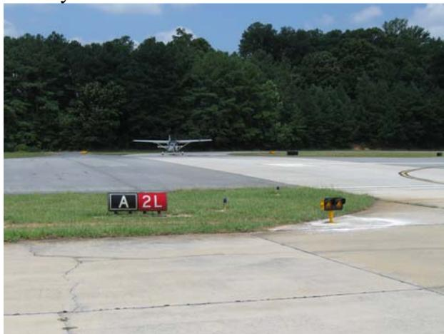
Additionally, there is a red & white runway warning sign that has been installed on the left side of the runway hold bar marking at the approach end of Runway 02Left. This on-the-pavement sign has been located on the left side of Taxiway ‘A’ to bring further attention to the upcoming, nearby runway and the hold short line for the Pilot-In-Command sitting on the left side of the taxiing aircraft.
