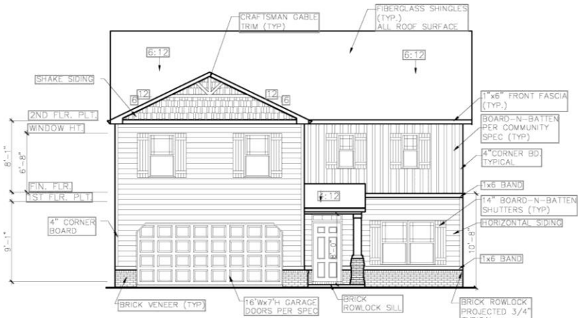
FRONT ELEVATION B2-3 (SCALE: 3/16"=1'-0")
