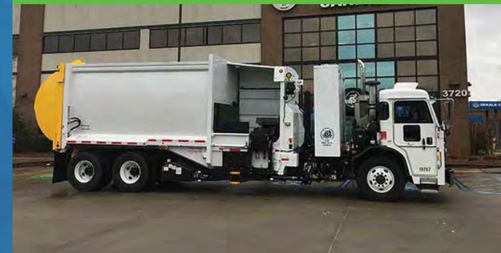
Sanitation Division Automated Side-loader (ASL) Truck
