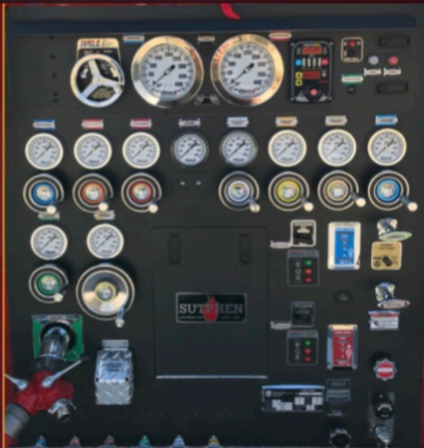
Engine pumper controls for charging hoses and flowing water .
