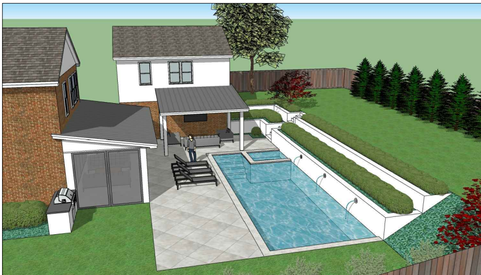
PROPOSED POOL, RETAINING WALLS AND POOL CABANA RENDERING - WALLS TO BE STUCCO - PAINTED TO MATCH HOUSE. SHOTCRETE POOL WITH PEBBLE-TEC PLASTER FINISH AND LIMESTONE POOL DECK.
