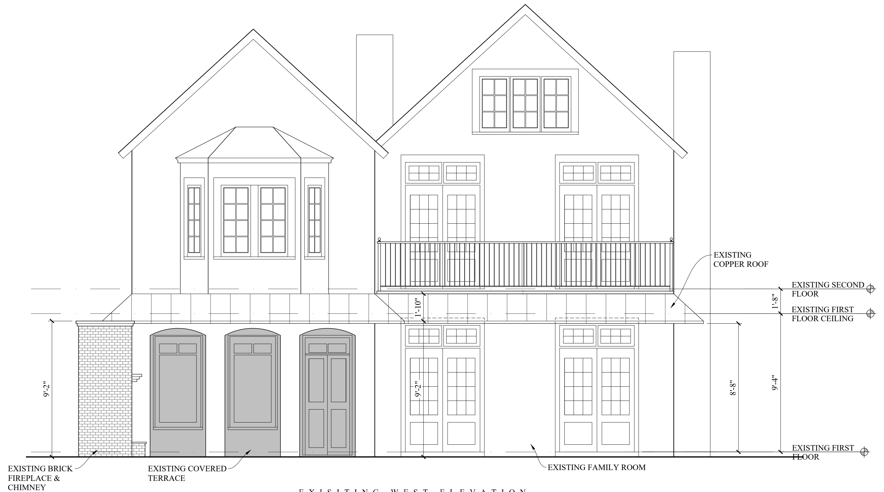
EXISTING WEST ELEVATION
