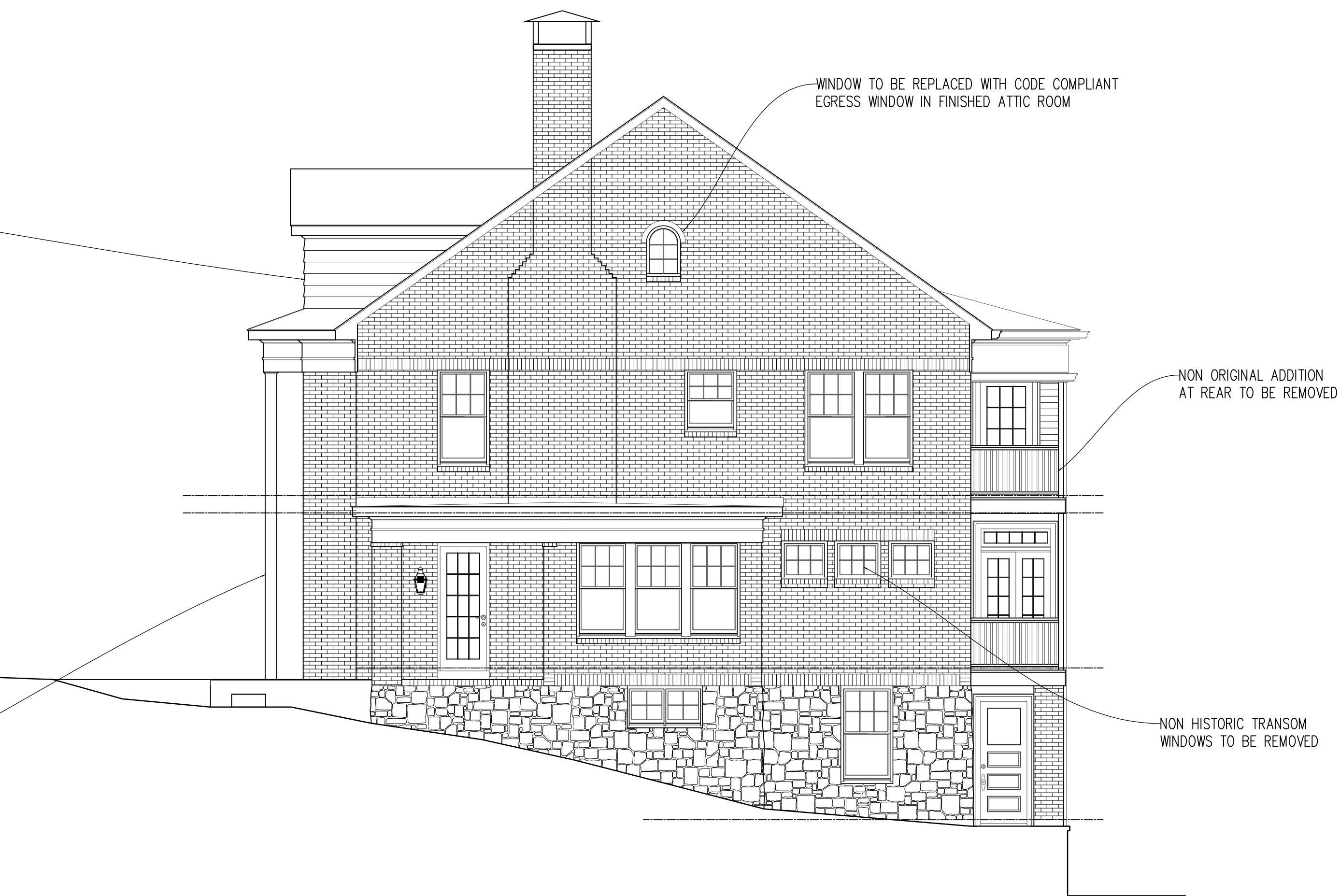
2 A-3 EXISTING DRIVEWAY SIDE ELEVATION 3/16"=1'-0"
