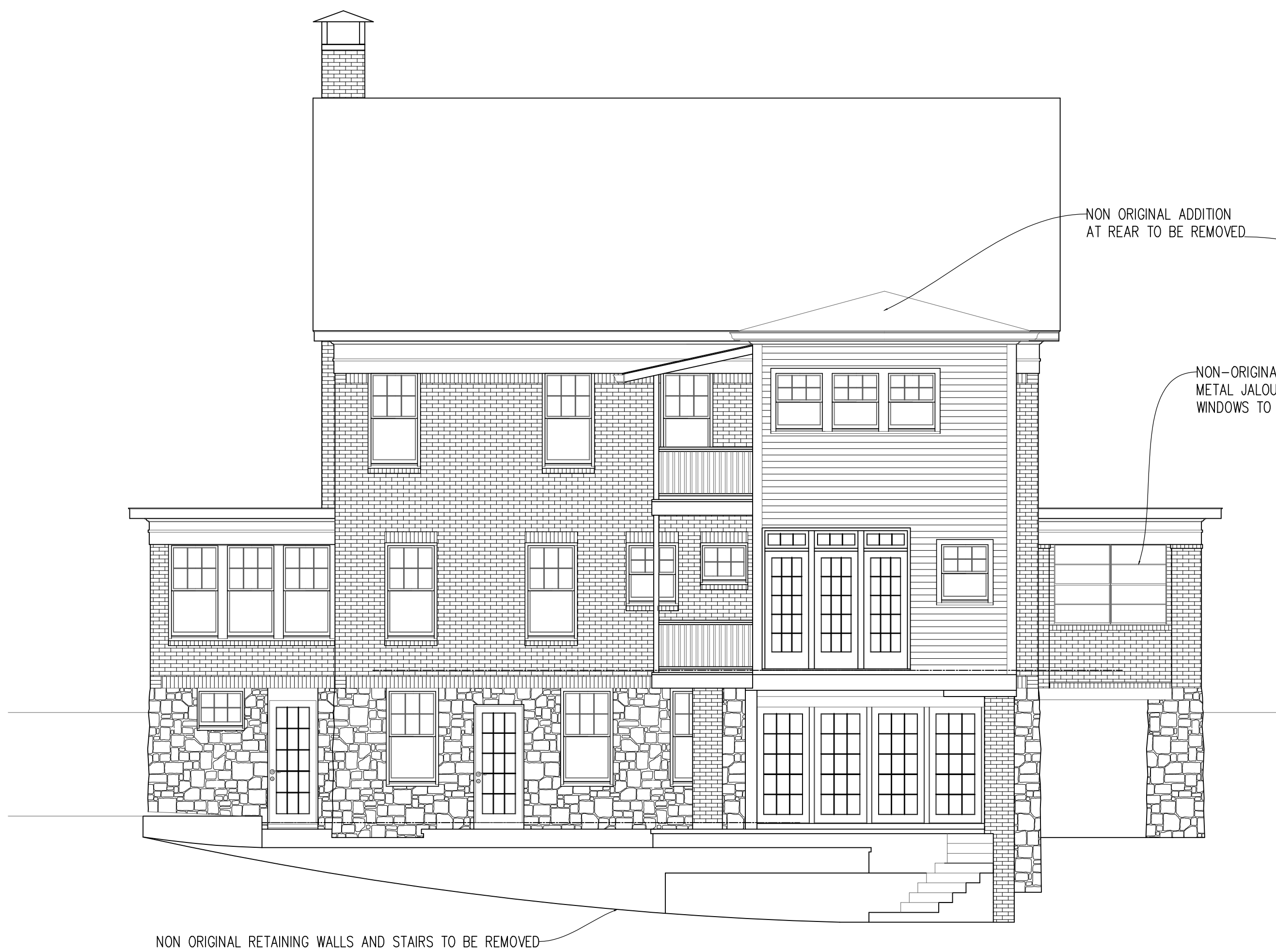
1 A-4 EXISTING REAR ELEVATION 3/16"=1'-0"
