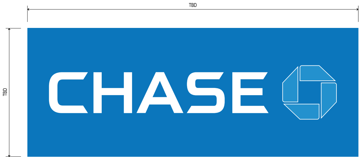
MT-A-V ACRYLIC FACE W/ LOGO AS VINYL 1ST & 2ND SURFACE SCALE: NTS Both Sides of Pylon to be Refaced
