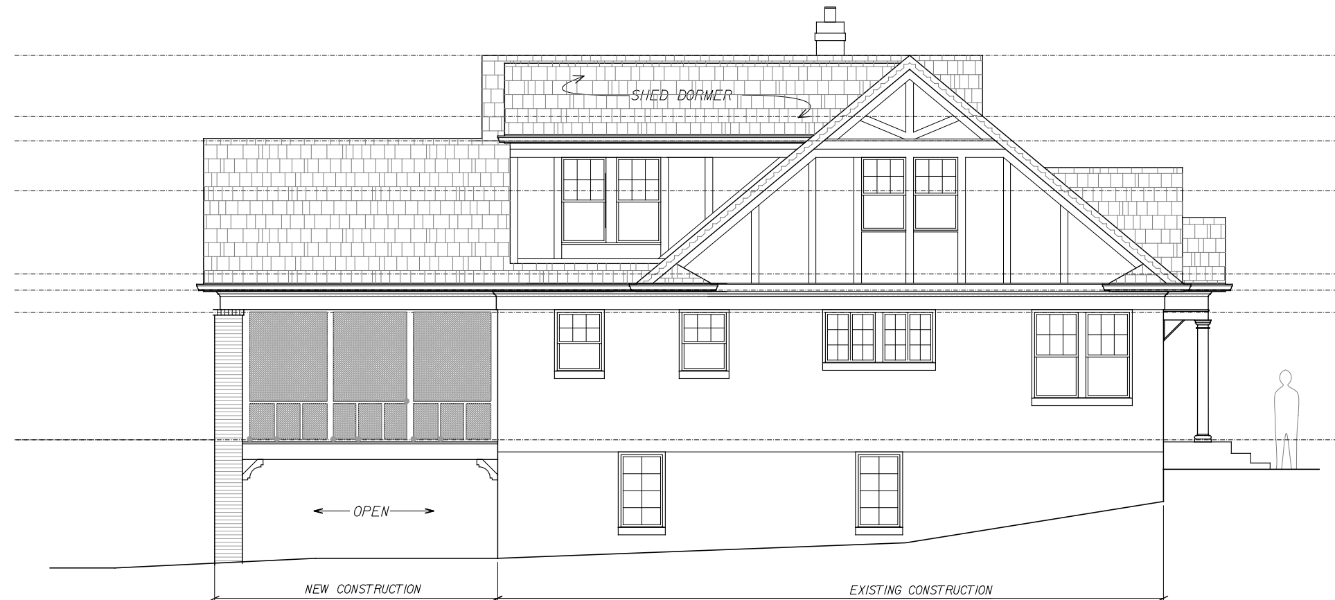
02 PROPOSED SIDE ELEVATION A-1.06 SCALE: 1/8" = 1'-0"
