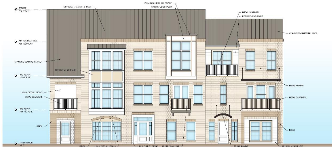
A TOWNHOME FRONT ELEVATION A - 2 CAR SCALE: 3/16" = 1'-0"
