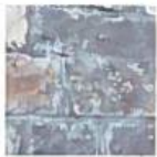
STONE WATERTABLE BISON STONE SUPPLY SANDSTONE, BATTERED APPROXIMATELY 8" H x 24" L COLOR: GREY RANGE
