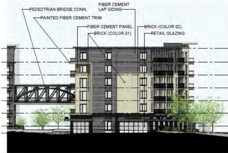
ELEVATION 5 - BUILDING A
