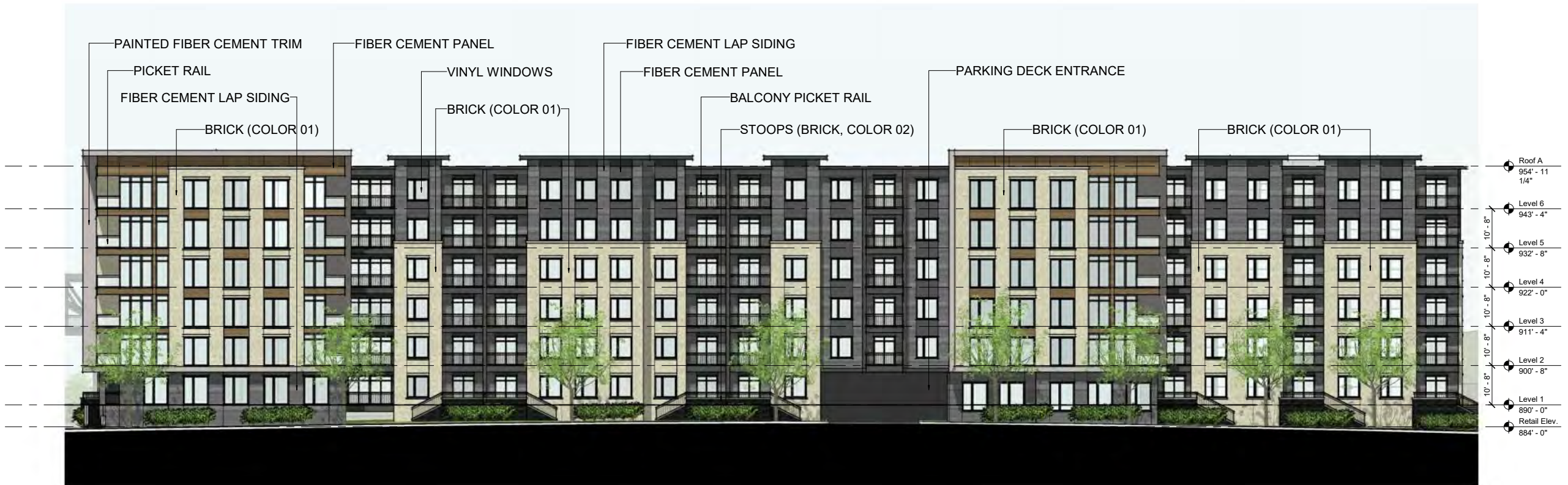
ELEVATION 7 - BUILDING B (CLAIRMONT RD)
