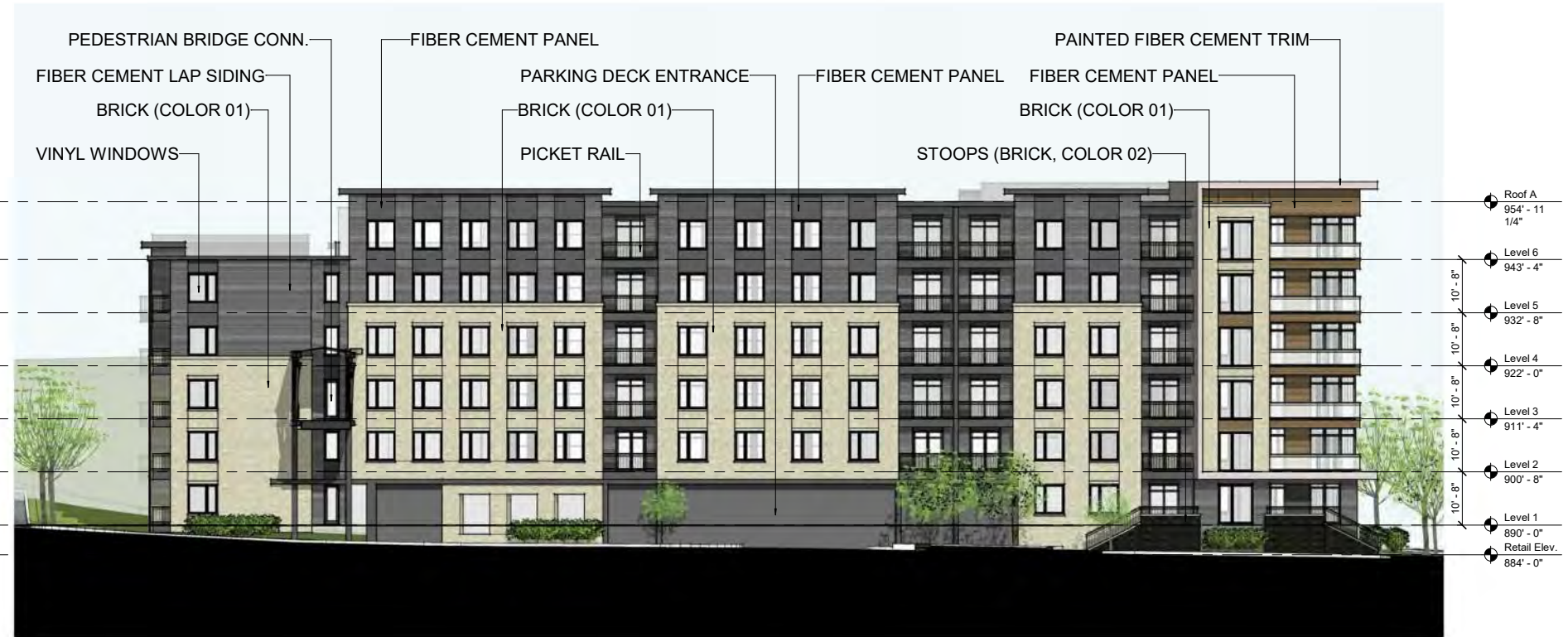
ELEVATION 6 - BUILDING B
