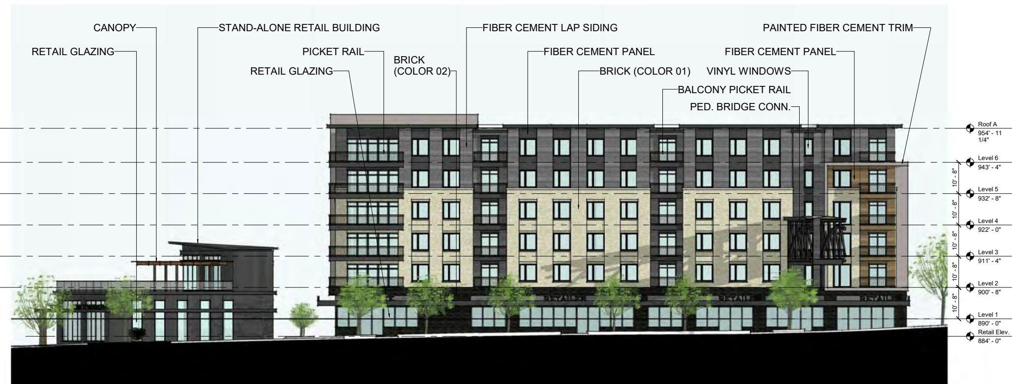
ELEVATION 4 - BUILDING A
