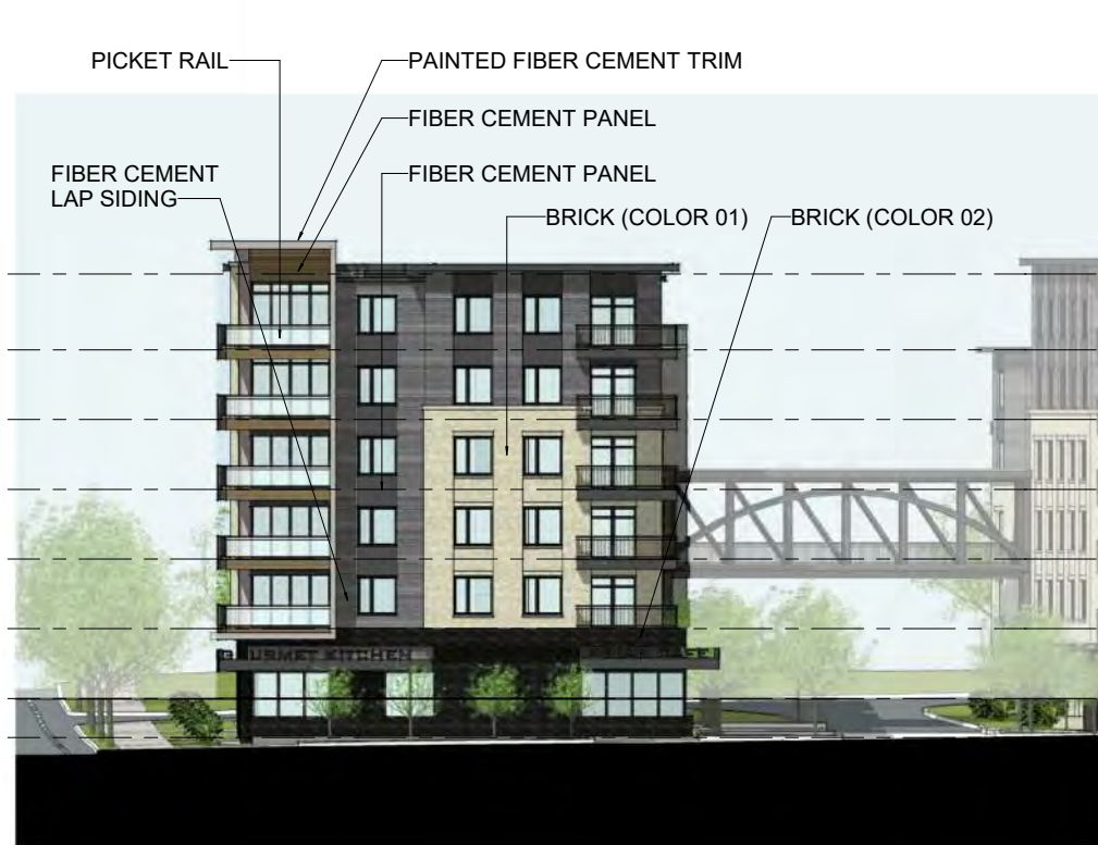
ELEVATION 1 - BUILDING A
