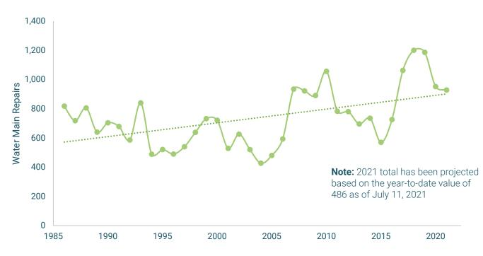
The increase in water distribution system failures results from two main causes: (1) aging pipelines and (2) excessive pressures on an under-sized system. CIP 2021 investments will target these issues.
